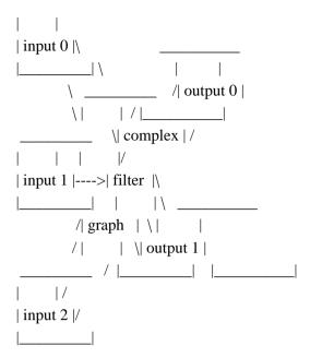
Complex filtergraphs are configured with the **-filter\_complex** option. Note that this option is global, since a complex filtergraph, by its nature, cannot be unambiguously associated with a single stream or file.
