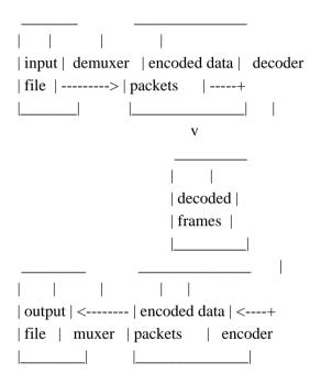
**ffmpeg** calls the libavformat library (containing demuxers) to read input files and get packets containing encoded data from them. When there are multiple input files, **ffmpeg** tries to keep them synchronized by tracking lowest timestamp on any active input stream.
