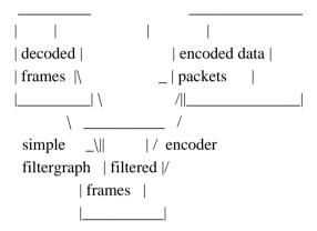
Simple filtergraphs are configured with the per-stream **-filter** option (with **-vf** and **-af** aliases for video and audio respectively). A simple filtergraph for video can look for example like this:
